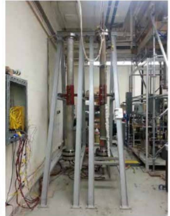
High Pressure, High Temperature Facility for Natural Circulation Experiments, City College of New York , NEUP Project 11-3218, Kawaji)
