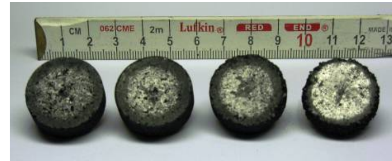
Oxidation/Degradation of graphite samples
