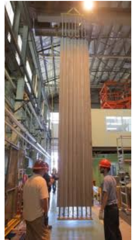
Finned water-cooled riser channels in the NSTF
